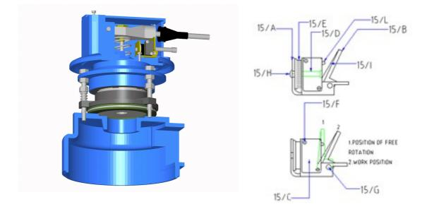
After having correctly performed the installation and regulation of the electric disengaged , with the brake of the motor still closed , the mobile anchor 15/B are prevented by the lever of unblocking 3 , to close the micro switch.
